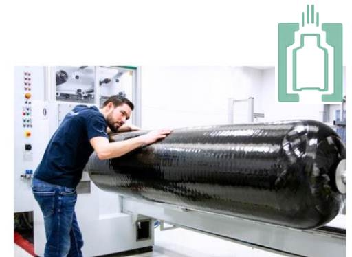
Kautex Maschinenbau Kautex has produced a 320 litre hydrogen liner through blow moulding.
